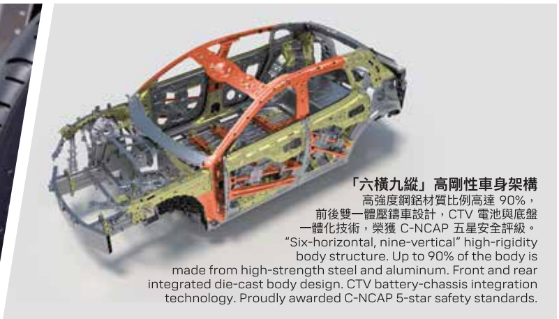
「七宮格」超長吸能門檻樑 1,968mm 超長保護範圍。 "Seven-grid" ultra-long energy-absorbing side beam delivers 1,968 mm of extended safety protection.
